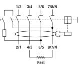
The value of the external resistance ( $\Omega$ ) depends on the I $\Delta$ n of the selected RCCB, as shown in the table:
