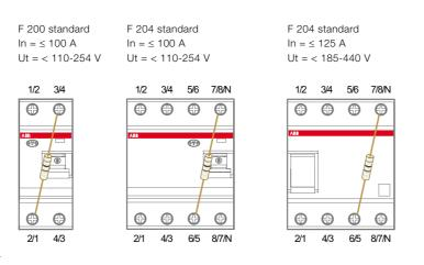
With this information, referring to the F202 standard it is clear indicated that the device will properly work if it is supplied between 110 and 254V.
