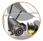
An indirect contact refers to a person coming into contact with an exposed conductive part which is not normally alive, but has become alive accidentally (due to insulation failure or some other cause). The protection against indirect contacts is mainly realized by disconnection of the supply, by means of a residual current device.
