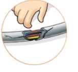
A direct contact refers to a person coming into contact with live parts or conductors that are normally live: the main protection against direct contacts is the physical prevention of contact with live parts by means of barriers, insulation, inaccessibility, etc.
