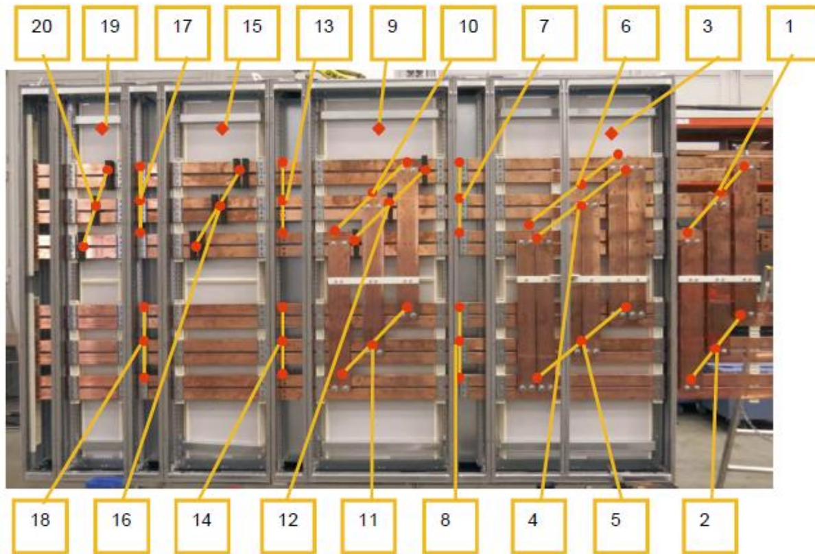
Diagram 5: Arrangement of selected temperature-measuring points along the main busbar
