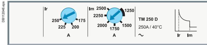
Circuit breakers equipped with thermal-magnetic trip units are used mainly in industrial and commercial electrical distribution applications:
