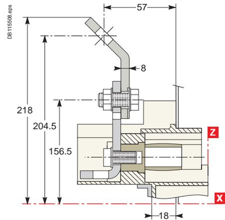
Double-L extensions: mounting on backplate (M) or rails (V)
