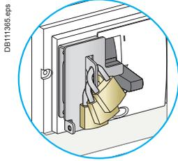
Fixed device attached to the case.
