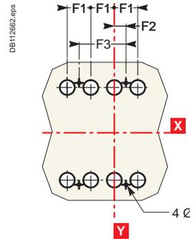
(1) The ØT1 holes are required for rear connection only (for two-pole circuit breakers, the middle holes are not required).
