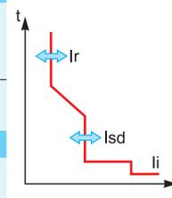
**(1)** If the trip units are used in high-temperature environments, the Micrologic setting must take into account the thermal limitations of the circuit breaker. See the temperature derating table.
