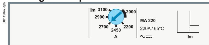
In distribution applications, circuit breakers equipped with MA magnetic-only trip units are used for:
