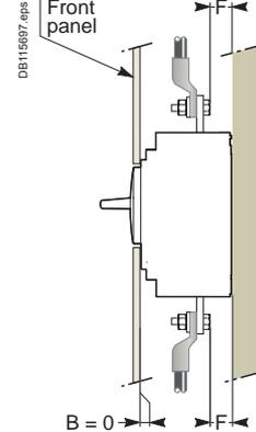
Bare or painted sheetmetal **Note:** if  $F < 8$  mm: an insulating screen or long terminal shield is mandatory (see page A-71).
