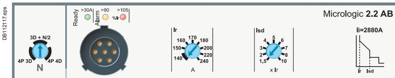
Compact NSX circuit breakers equipped with Micrologic AB trip units are installed as incoming devices for consumer installations connected to the public LV distribution system.
