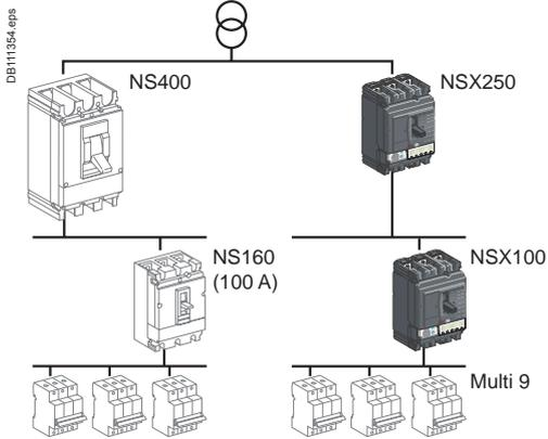
**Compact NSX100 with Micrologic for total discrimination with Multi 9 devices rated  $\leq 40$  A or a C60. Better coordination between protection functions reduces the difference in ratings required for total discrimination.**
