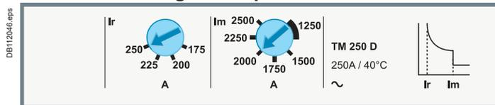
The 16 Hz 2/3 frequency does not modify the thermal settings with respect to those at 50 Hz (see page A-13). The magnetic pick-ups are modified as shown below.
