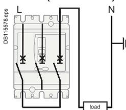
Remark. For an operating voltage > 250 V, the installation must be designed to eliminate all risk of double earth faults.
