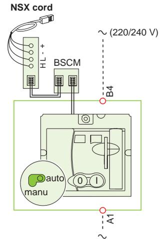
**Communicating motor mechanism (MTc)**
