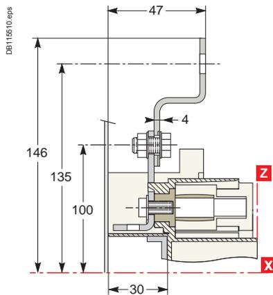
Double-L extensions: mounting through front panel (N) or on rails (V)
