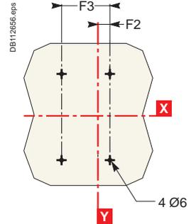
**Connection by exterior-mounted rear connectors**
