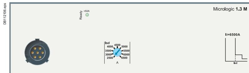
Micrologic 1.3 M trip units provide magnetic protection only, using electronic technology. They are dedicated to 400/630 A 3-pole (3P 3D) circuit breakers or 4-pole circuit breakers with detection on 3 poles (4P, 3D) and are used in certain applications to replace switch-disconnectors at the head of switchboards. They are especially used in 3-pole versions for motor protection, see page A-38.
