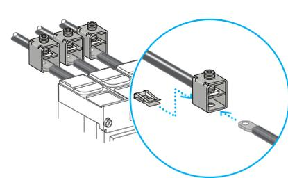
Connection of bare cables to NSX100 to 250.
