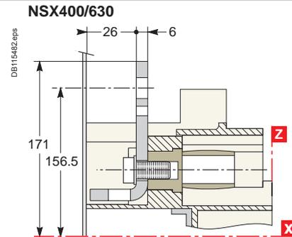
Rear connection: mounting through front panel (N) or on rails (V)
