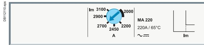
Circuit breakers with an MA trip unit are combined with a thermal relay and a contactor or a starter.
