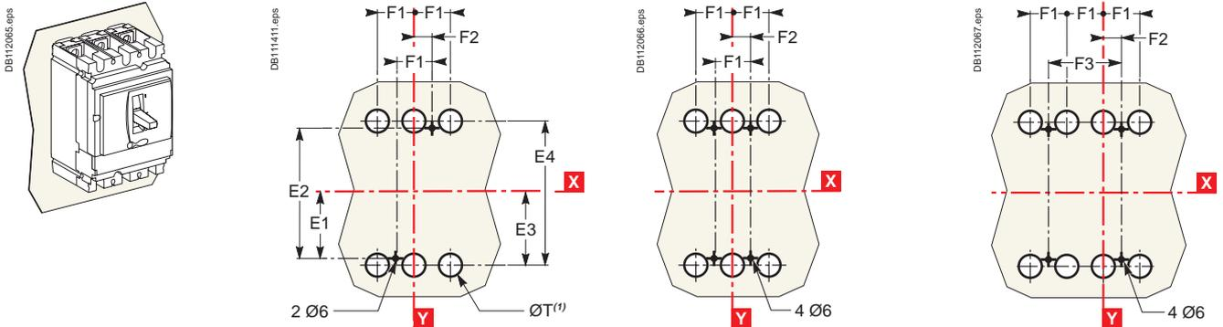
(1) The  $\text{ØT}$  holes are required for rear connection only.
