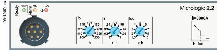
Circuit breakers equipped with Micrologic 2 trip units can be used to protect distribution systems supplied by transformers. For generators and long cables, Micrologic 2 G trip units offer better suited low pick-up solutions (see page A-48).
