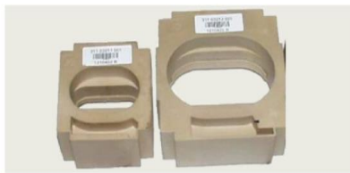
Current sensor is a Rogowski coil. Rogowski coil is not saturated compared to iron core current converters and has exact measurement!
